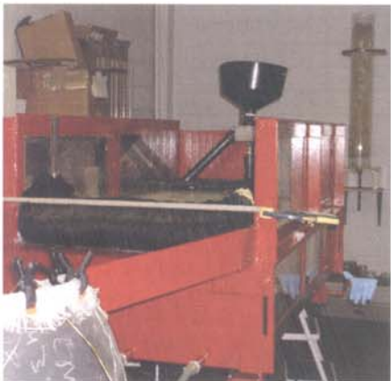
Fig. 1: Flume for flow rate testing.
