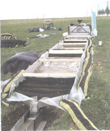
Fig. 2: Example of field experiment setup for three sets of socks, with five socks in each set.
